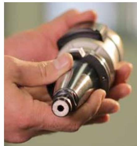
Example of a toolholder with a coolant hole
